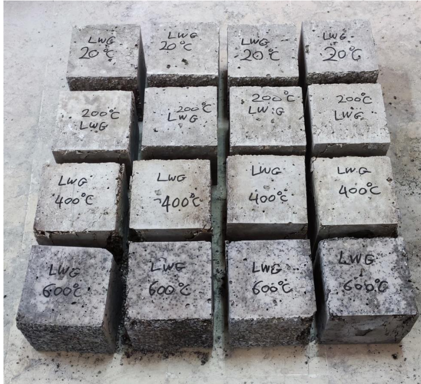
Figure 4: Color appearance of LWGC specimens exposed to elevated temperatures
