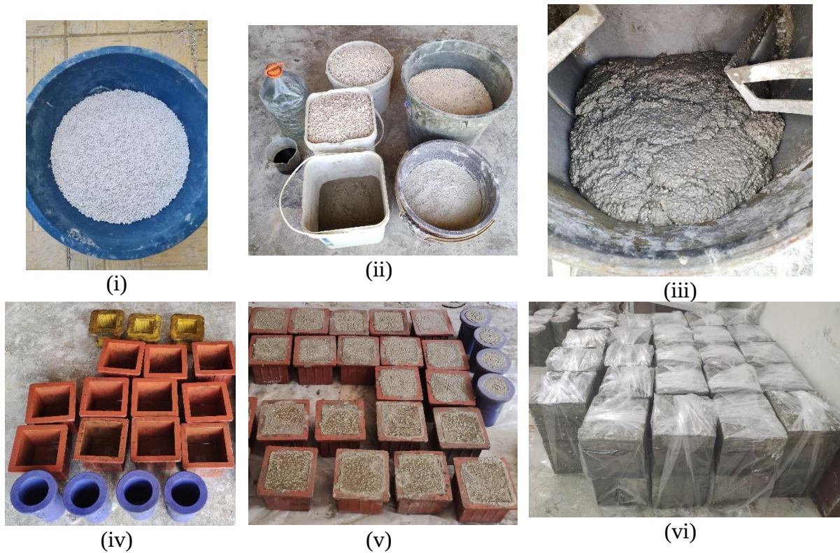
Figure 1: Mixing, casting, and curing of the LWGC samples: (i) EGGA; (ii) consistent ingredients; (iii) blending activator with geopolymers; (iv) molds used for casting specimens; (v) casting and vibration; (vi) specimen curing
